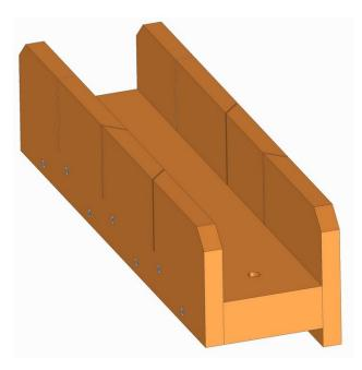
The kerf for the saw to run in should be made with a back saw or a panel saw. For cutting the kerf you should use the same saw that you will normally use for mitreing.
