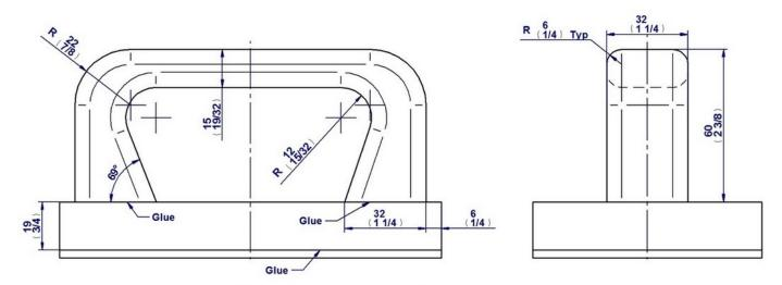
The glue joints are long grain to long grain - screws are not needed
