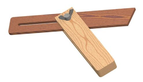
Sliding T bevel consists of a stock (or handle) and a slotted blade (or tongue) that pivots on a machine screw with wing nut. The blade may be fixed firmly at any desired angle by simply turning the wing nut (or knurled screw). Use the dimensions in the plan as guidance; in case you need some dimensions that are different from those given in our plan, simply adjust the sliding T- bevel to the dimensions that suit you.
