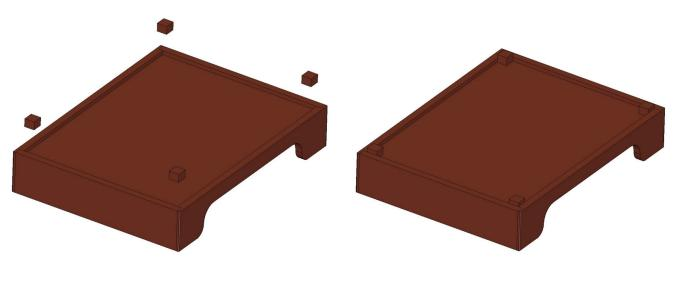
3. Fasten the Decorations (part 6) on the subassembly corners made in previous step. Use the Tacks D1,4  $\times$  8mm (parts 7) for this procedure.
