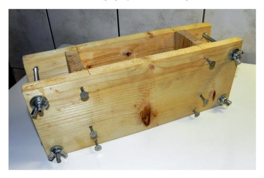
For easier assembly of the mold after use, mark the position of parts with a pencil so that you can always put them back to the position in which the nail holes overlap.
