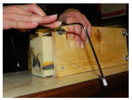
For this purpose it is necessary to remove the bottom part, one side part and a set of lower fasteners, and slightly loosen the remaining three fasteners so that the soap block could be moved in the mold. Once the end of soap loaf is taken out of the mold, the thickness of the cut pieces is defined (we suggest 2.5 cm / 1''), and the edges of the mold sides then serve as a slot for guided cutting.
