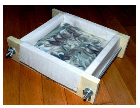
The slab mold plan presented here has internal dimensions of  $17 \times 17$ cm (6.7 x 6.7"), which is enough for 6 soaps of size 8.5cm x ca. 5.6cm (3.3 x 2.2"). Mold cavity depth is 5.4cm. For a soap thickness of 2.5cm (1") in this mold you need a batch made from 550g (19.4oz) of oil. If you want to use dividers, make them of solid but thin plastic. If you use thicker plastic, increase internal size of mold by as many mm as are taken by the dividers (e.g.  $18 \times 18$ cm).
