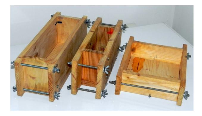
The molds are designed in such a way that they are fully and easily demountable, and different sizes can be assembled by combining of parts. Depending on the desired soap dimensions and how many bars of soap you want to get from one batch, you can calculate the needed mold dimensions. Our plan can be easily adjusted to your needs.
