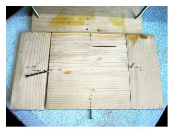
It is important that all the sides of the parts are flat, well-sanded, and fit well with one another as this minimizes the risk of leaking liquid soap batter after pouring.
