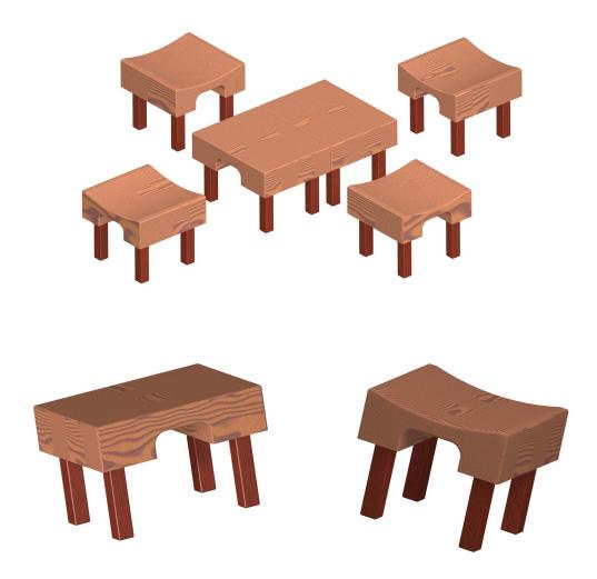
In the drawings you can see the layout and dimensions of all parts, the drawing and exploded view of the assembly, and the parts list. All parts are interconnected by gluing, and the axle part is optional – even if you choose not to use it, the adhesive will provide sufficient strength to all existing joints in the tables and chairs. If it is easier for you, make the legs with a circular cross-section.
