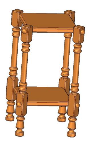
As you can see in the picture, here you are offered a plan to build a tabouret stool that consists of four legs and two boards. The legs and boards are interconnected with the parts named pins. These pins are in fact dowels with a rounded head, which have a decorative role.
