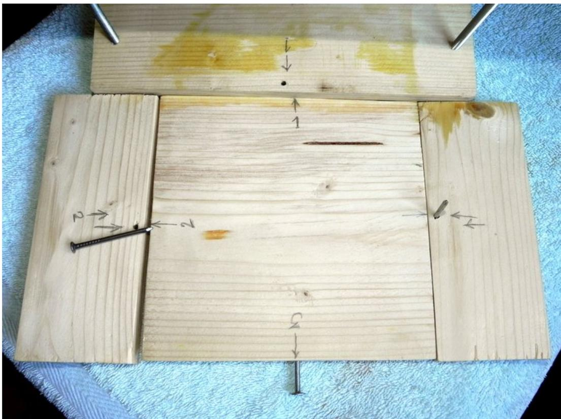
It is important that all the sides of the parts are flat, well-sanded, and fit well with one another as this minimizes the risk of leaking liquid soap batter after pouring.
