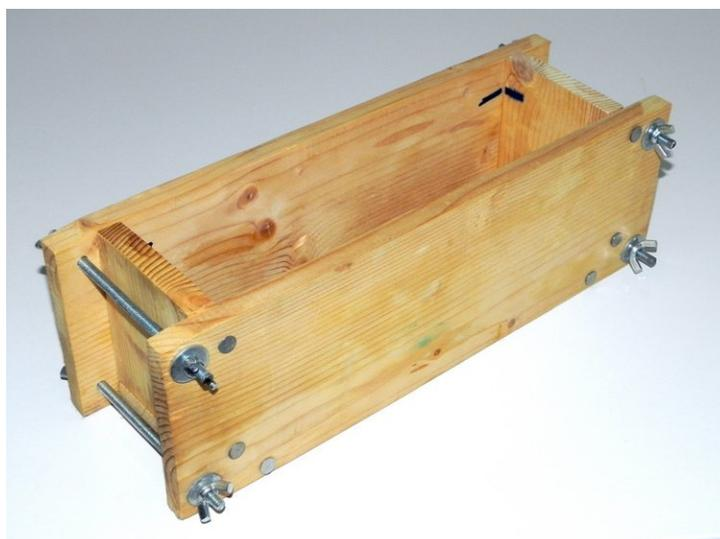
This loaf mold is similar to tall skinny log molds, the only difference is the width of the finished soap. In the following picture you can see how the soaps look like in each of the molds.
