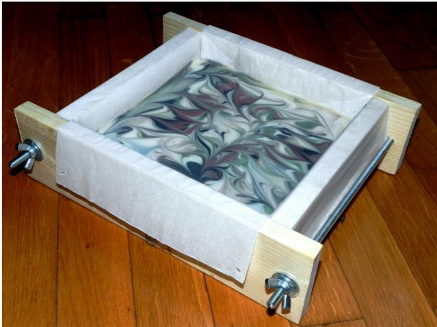
The slab mold plan presented here has internal dimensions of 17 x 17cm (6.7 x 6.7"), which is enough for 6 soaps of size 8.5cm x ca. 5.6cm (3.3 x 2.2"). Mold cavity depth is 5.4cm. For a soap thickness of 2.5cm (1") in this mold you need a batch made from 550g (19.4oz) of oil. If you want to use dividers, make them of solid but thin plastic. If you use thicker plastic, increase internal size of mold by as many mm as are taken by the dividers (e.g. 18 x 18cm).
