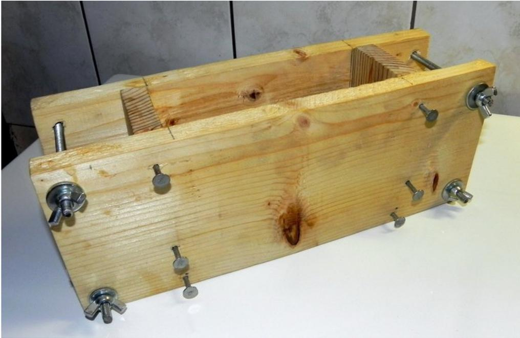
For easier assembly of the mold after use, mark the position of parts with a pencil so that you can always put them back to the position in which the nail holes overlap.
