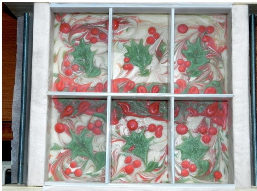
In order to assemble the mold, neither woodworking joints nor glue are used due to the necessity that the mold is completely demountable, and that its demounting can be done easily, quickly and in just a few moves. The mold is mounted with fasteners (Threaded rod M4, Wing nut M4 and Washer). By turning the wing nut, the mold becomes compact enough for use. For proper placement of holes, both side parts need to be drilled in one session.
